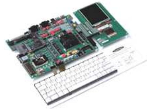
Aiji System SMDK2410 •Samsung S3C2410 •Accepts Smartmedia Cards
