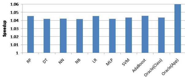
Figure 4. Program improvement with the prediction models. The comparison baseline is the optimal suite-level optimizations.
